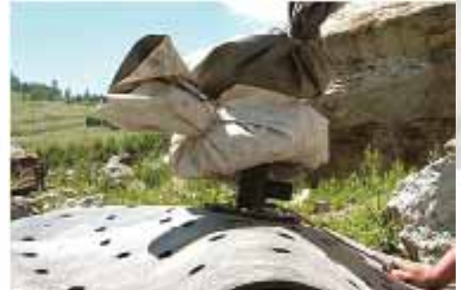
10 The Rock Cracker is loaded with sandbags to provide weight.
