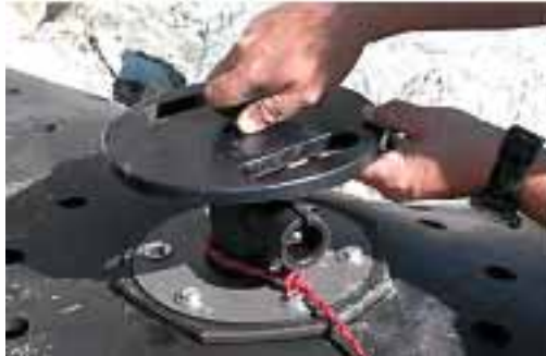
9 A loading plate is screwed on to the firing mechanism.
