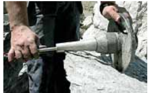
14 The starter is removed again with the aid of a cartridge ejector.
