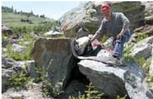
13 The result: The block was split successfully into several pieces with the Rock Cracker.
